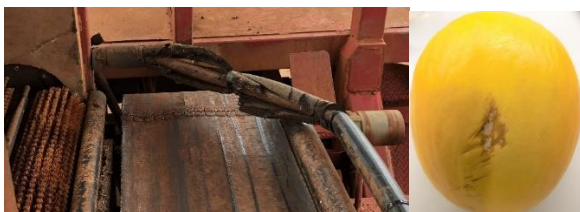
Image 5: Worn padding on harvest equipment (left) and impact damage on a specialty melon (right).
