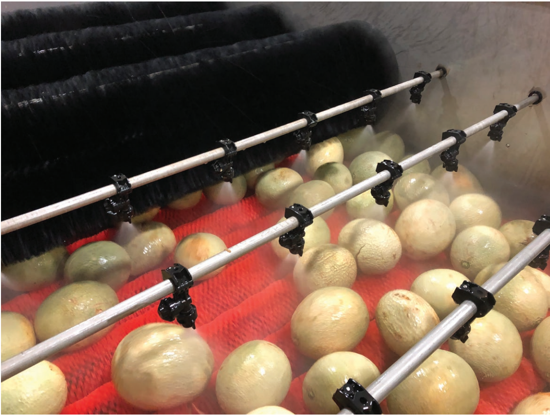
Figure 28. Rockmelons being washed, brushed and sanitised under a spray bar system.
