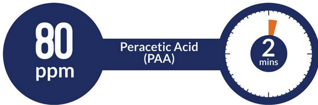
Figure 36. For washing and sanitising rockmelons and specialty melons, 80 ppm concentration of PAA with a minimum two minutes contact time is recommended.
