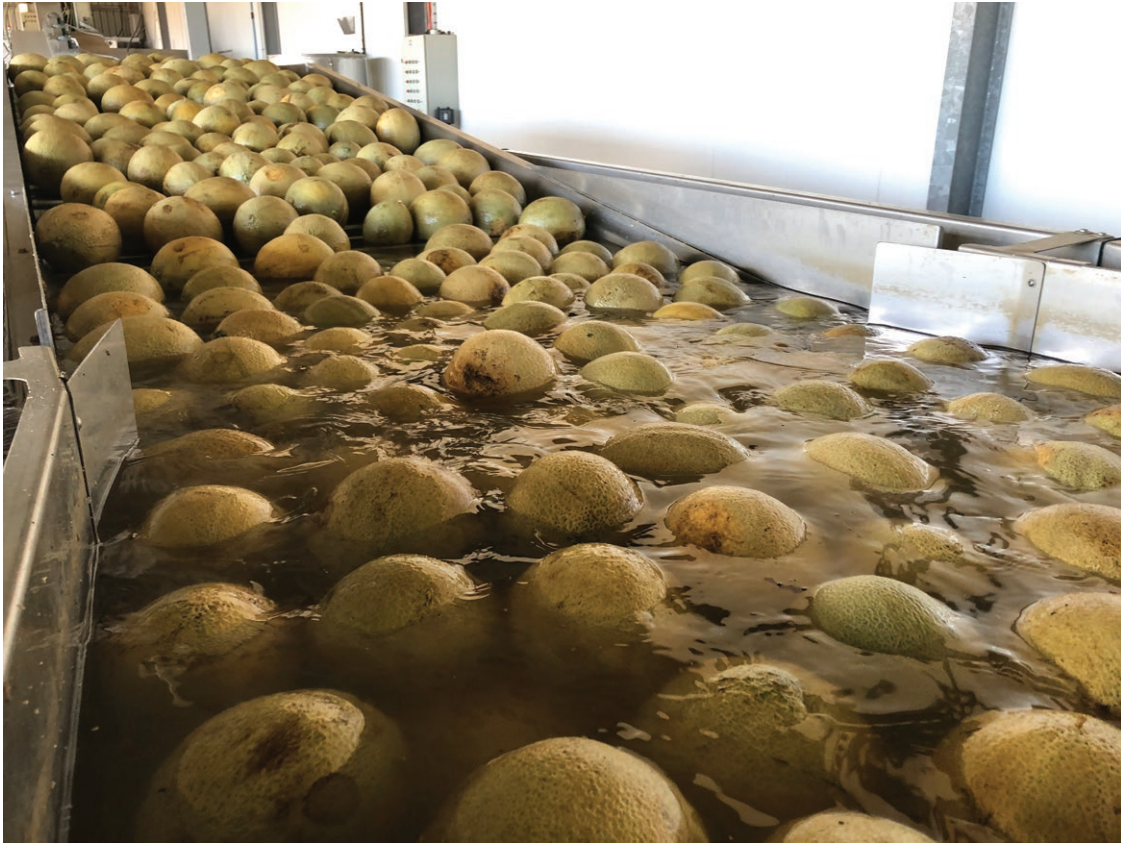
Figure 21. Wet dumping: the fruit is placed directly into large capacity tanks containing sanitised water.
